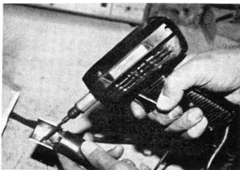
Closeup of Rocklin Beamed Thunderbolt Gun using tungsten carbide electrode being applied to bore area of worn collet pad.
